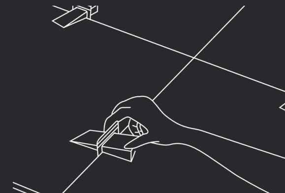
The contributing factors to what causes TechnoSLAB lippage are how much warpage the TechnoSLAB has, the width of the grout, how flat the substrate is, and the expertise of the tile installer. We recommend that lippage should not be greater than 2mm at the most for this type of installation.
