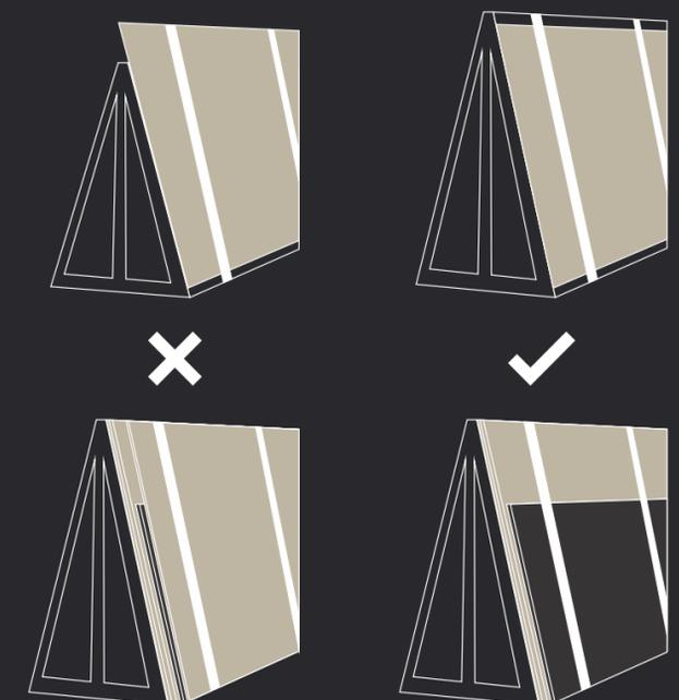
Avoid positioning large slabs against smaller slabs:
