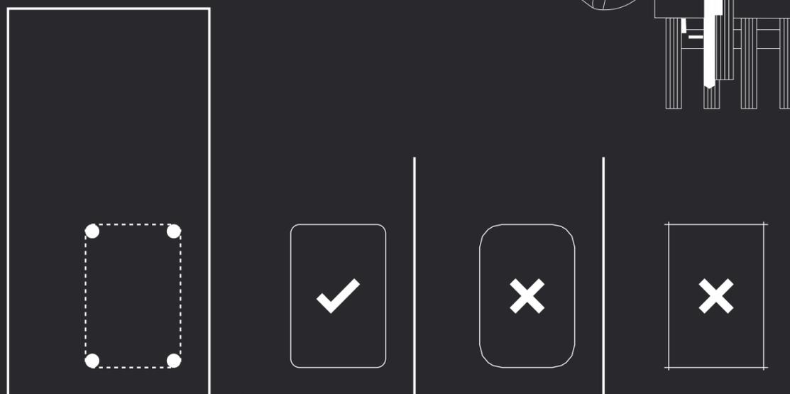
Prepare the holes on all inner corners, minimum 3mm bit diameter.
