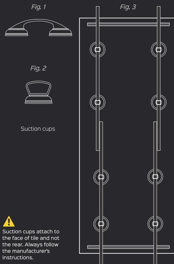
Typical suction cups (Fig. 2) of different kinds are a prime aid, although a couple of workers will be needed to carry the tiles and these may still get deformed.
